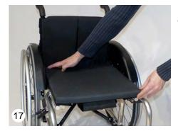
• Press the seat cushion equally and firmly on the nylon cover. (17)
