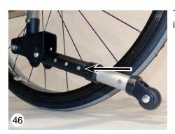
The length of the anti-tip is adjustable in three positions respetively in 2,5 cm steps (46).
