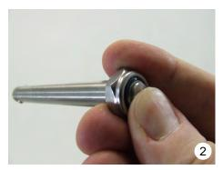
• Whilst pressing the release knob, position the quick-release axle into the rear wheel bearing (3).
