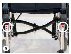
• Check also visually if the locking bolts are engaged (9).
