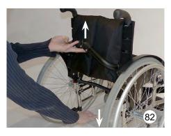
• Move the backrest cross bar to the top (82) and move the cable pull at the same time downwards (82).
