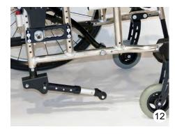
• To activate the anti-tip move the the anti tip with the foot downwards (13).
