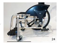
The **seat angle** depends on the chosen size of rear- and front wheels as well as the height of the rear axle and the position of the front wheels in the castor.
