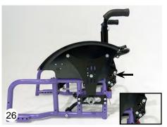
The **backrest angle** is from 80° up to 110° adjustable. **FARO** was built in accordance with the customer's order It is possible for the technician to modify the wheelchair with a different seat height.
