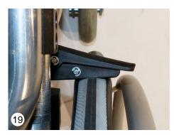
The brake shoe presses on the tires and grips it tightly. The brake shoe is, therefore, at a 90° angle to its holder (19). The brake shoe should overlap 3-5 mm to the middle of the wheel (19).
